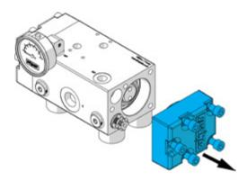
3. Remove water valves and O-rings.
