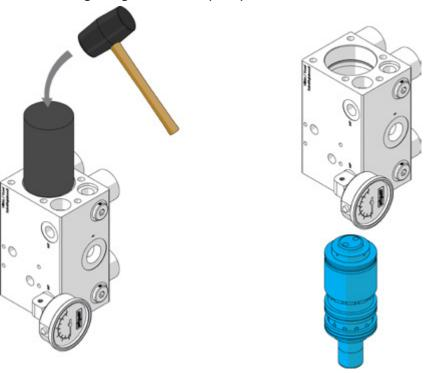
6. Remove the sealing flanges from the piston assembly.
