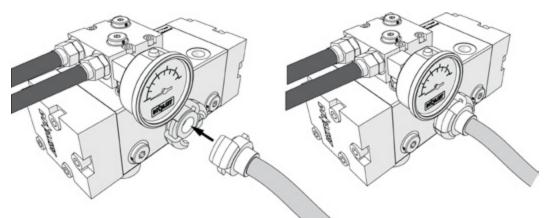
Picture 23: Connection to the pumping fluid intake
