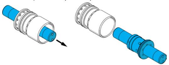
9. Remove seal from the piston assembly and o-ring from the cylinder.
