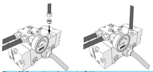
Picture 25: Connection to the pumping fluid output
