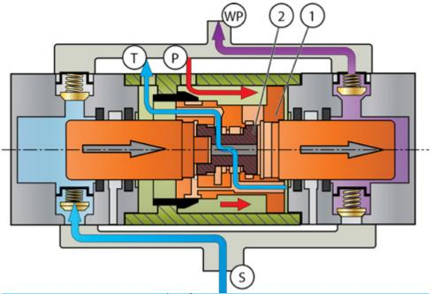
Picture 5: Operating principle of HDF pump 1
