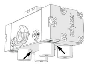
Picture 22: Leakage detecting bores
