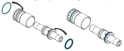
11. Install the piston assembly to the cylinder. Use vaseline or mineral oil to the seal and mating surfaces to make installation easy.
