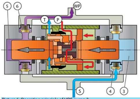
Picture 6: Operating principle of HDF pump 2
