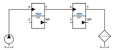
Picture 9: HDF hydraulic line connection in series
