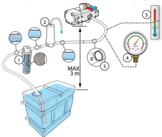
Picture 24: Installation into pumping fluid line
