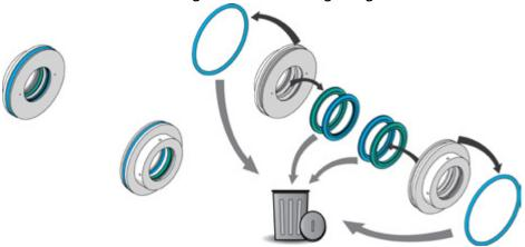
8. Remove the piston assembly from the cylinder.
