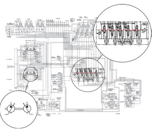
Picture 10: Open centre hydraulic system with Load Sensing variable displacement pump
