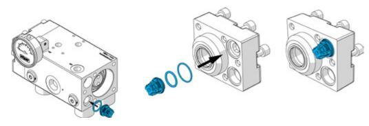
5. Install the head. Tighten heads bolts across, READ CHAPTER "6.6. Bolt tightening torques"
